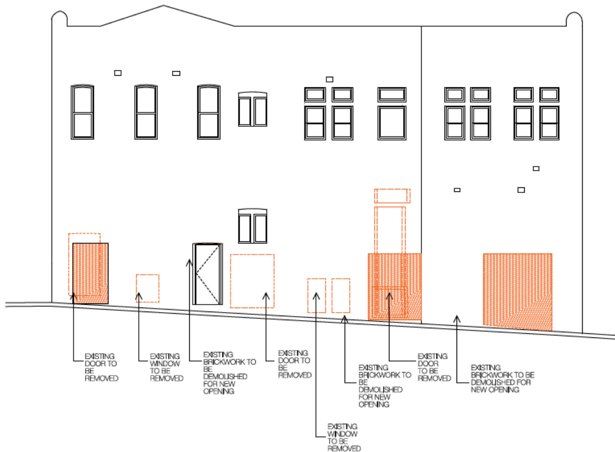
Patterson Lane (south) elevation demolition plan
